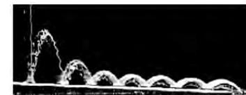
Figure 6 Bouncing water droplet on Nano-turf. The mass of the droplet is around 5 mg and the inclination of the nanoturf is 3.9°.
